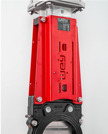
The robust metal yoke enables the optimal, simple assembly of mechanical or inductive limit switches. The yoke can be removed from one side. This makes it easier to access the mechanical parts.
