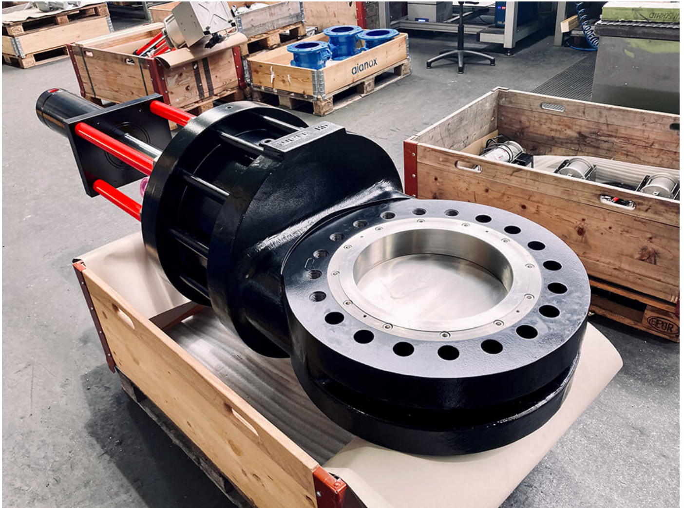
Wey HDH DN 350 at our production site in Switzerland.
