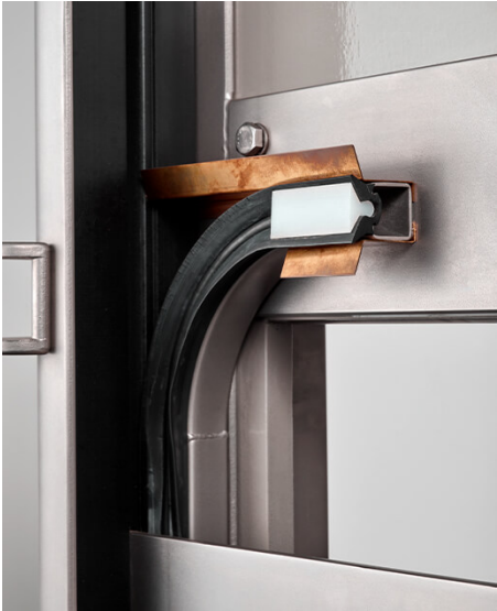
Seal with NBR, flush to the bottom, circumferential, easy to replace, transverse seal with double scraper.
